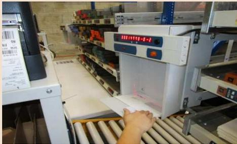
2. An indicator lights up in the compartment from which an item needs to be taken. And the quantity to be taken is shown on the pigeon hole display.
